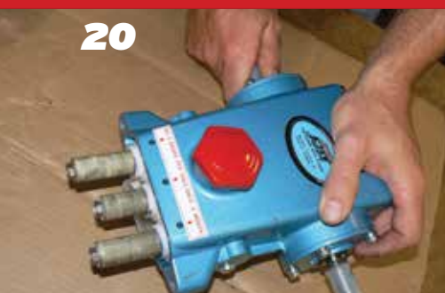
Inspect O-Ring and Back-Up Ring for wear & replace if needed. Examine Ceramic Plunger for scoring, scale build-up, chips or cracks and replace if needed.
