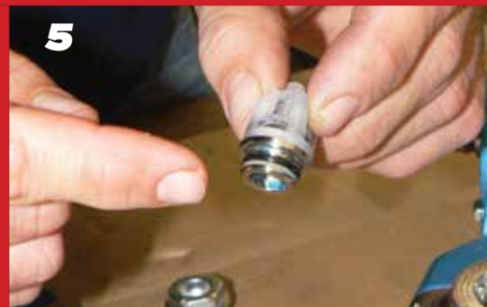
5 Examine the Valve O-Ring for cuts or distortion and replace if worn. Lubricate the new O-Rings before installing on the manifold.
