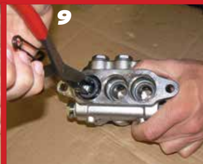
9 Hi-Pressure Seal is easily removed from the manifold without any tools. If extremely worn a reverse pliers may be used.
