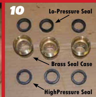
10 Correct Seal arrangement
