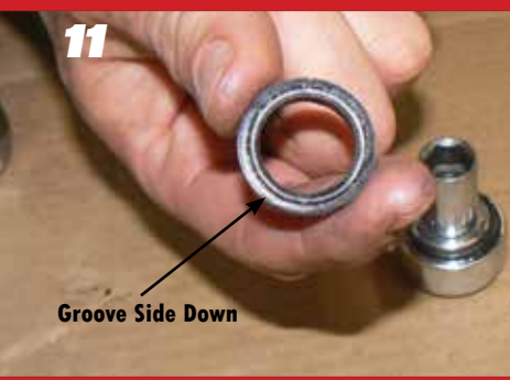
Carefully square Hi-Pressure Seal into position by hand with the grooved side down .
