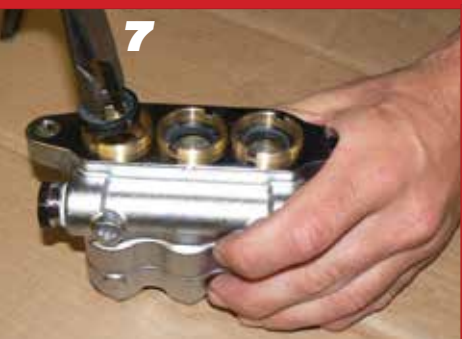
7 Place Manifold Head on work surface with crankcase side up . Remove Lo-pressure Seal On 5PFR & 7PFR plunger pumps prior to May 1989, remove Snap Ring & Lo-Pressure Seal from each Seal Case. Discard Snap Rings. On 5PFR & 7PFR plunger pumps after May 1989, remove Lo-Pressure Seal from each Seal Case.
