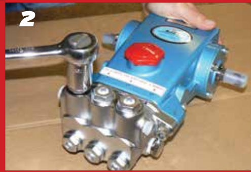
2 Remove the hex Valve Plugs (top discharge, bottom inlet)
