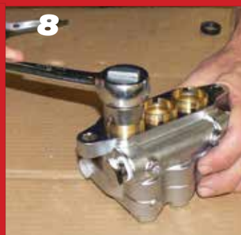
8 Remove Seal Case from each seal chamber. Remove O-Ring from outside diameter of Seal Case.
