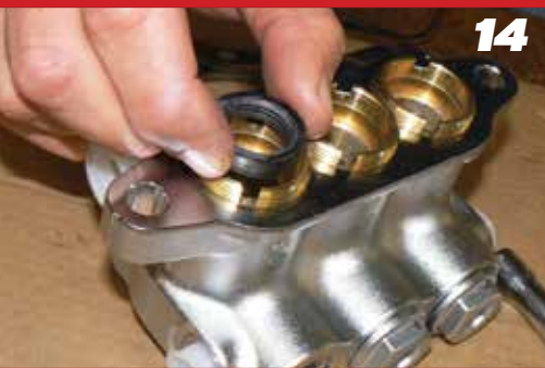
Install Lo-Pressure Seal into each seal case with Garter Spring down .
