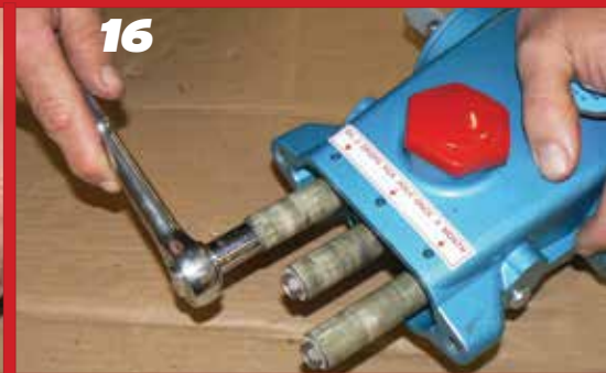
Using an M12 hex tool on the 5 & 7 pumps, loosen the plunger retainer about three to four turns.
