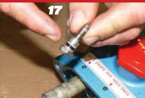
Inspect O-Ring and Back-Up Ring for wear & replace if needed. Examine Ceramic Plunger for scoring, scale build-up, chips or cracks and replace if needed.
